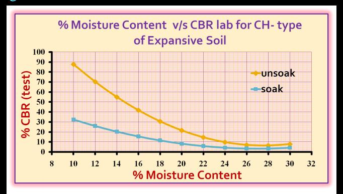
$\Box$  The value of *CBR* is directly determined from % Moisture Content and the figure shows the relationship. And it is applicable for the *CH*-type of compacted expansive soil only.
