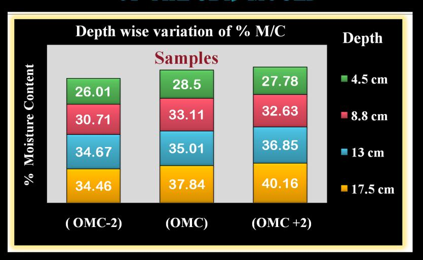
5) The unconfined compressive strength of compacted sample at OMC was 3.0 kg/cm<sup>2</sup>. C<sub>u</sub> is very sensitive to moisture content of compacted clay.
