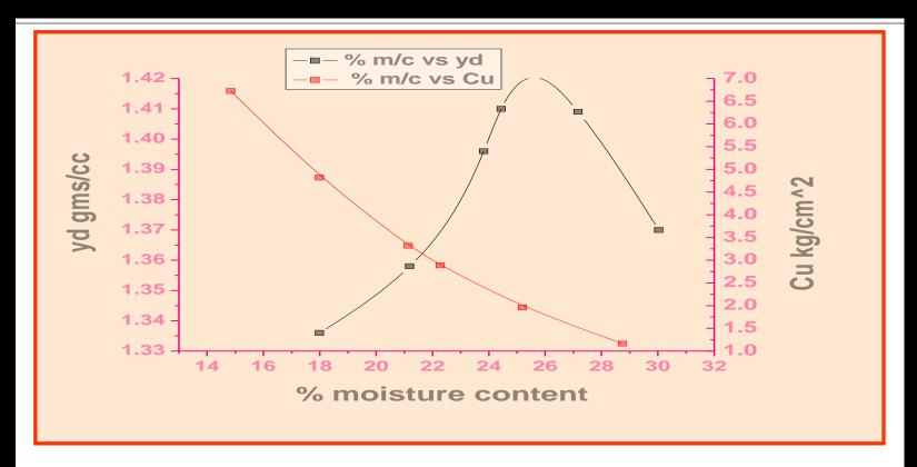
The value of  $C_u$  is determined by UCC test and the relation between % Moisture Content,  $\gamma_d$  and  $C_u$  is as shown in figure.
